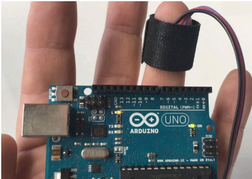
Photo of LED13 Blinking with a user's heartbeat.
